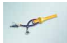
Wet sprayed concrete polyurethane spray gun
