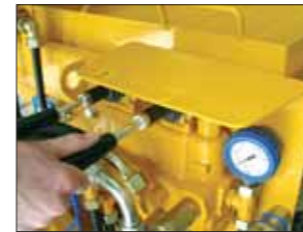
The screw pump may be readily operated in either forward or reverse, thus enabling the hoses to empty in case of clogging.
